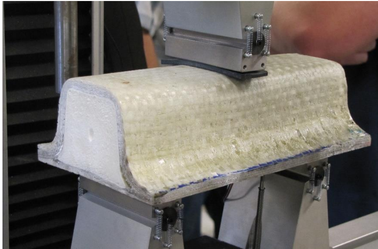
Figure 3.4: Type 3 (PRISMA FOAM) Sandwich Panel Specimen
