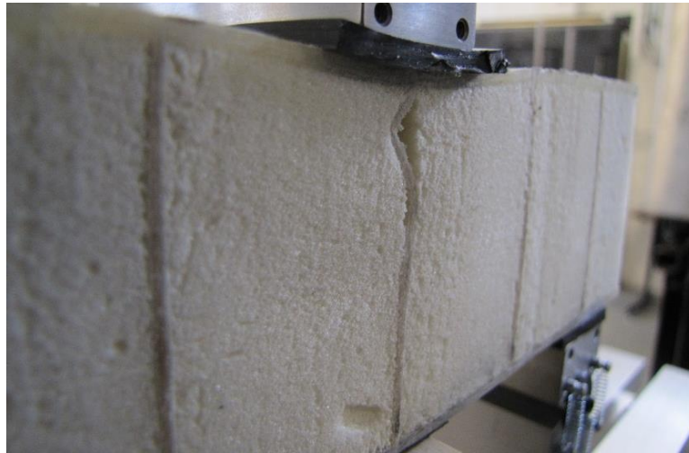
Figure 3.13: Initial Failure Due to Buckling of the Reinforcing Webs and Local Indentation for Type 2
