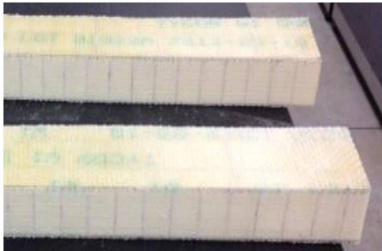
Figure 2.2: Type 2 Polyurethane Foam (WEB-CORE)
