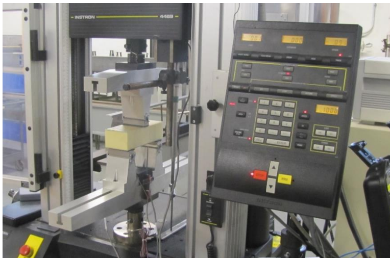
Figure 3.5: Three Point Flexural Test Setup
