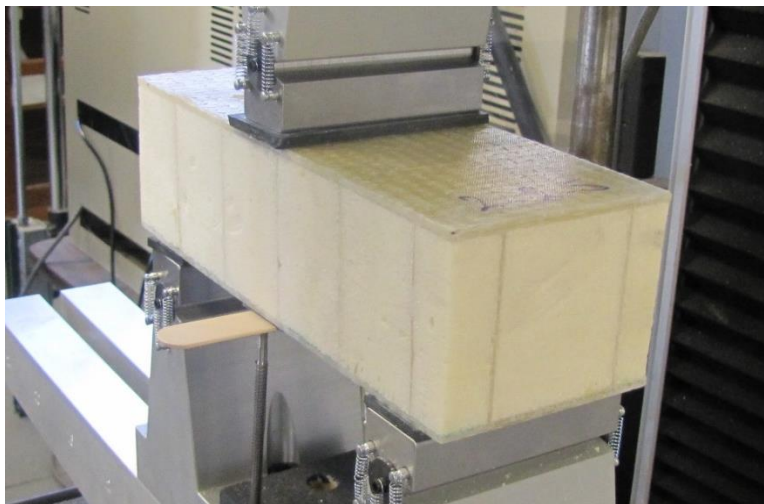
Figure 3.3: Type 2 (WEB-CORE) Sandwich Panel Specimen
