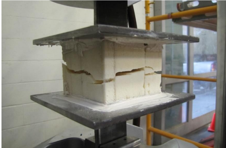
Figure 2.21: Type 2 Core Failure During Flatwise Tension Test
