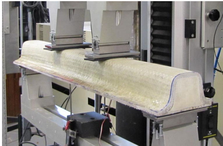
Figure 3.22: Type 3 (PRISMA FOAM) Sandwich Panel Specimen
