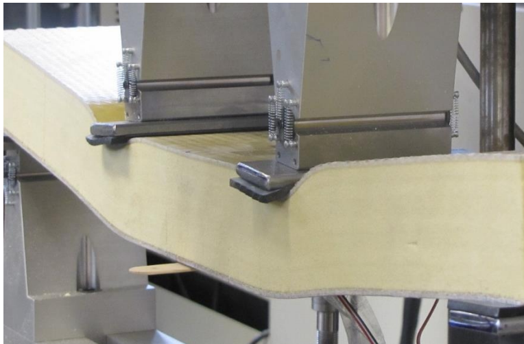
Figure 3.28: Ultimate Failure Due to Excessive Local Indentation for Type 1
