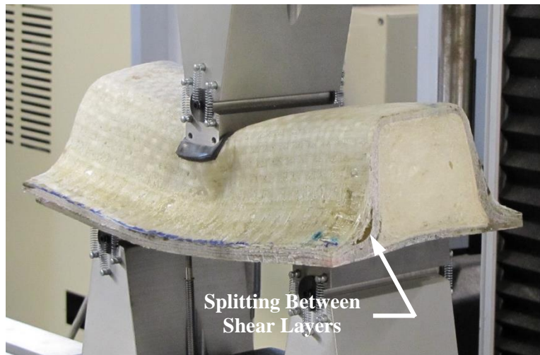
Figure 3.18: Ultimate Failure Due to Excessive Local Indentation and Splitting Between Shear Layers for Type 3
