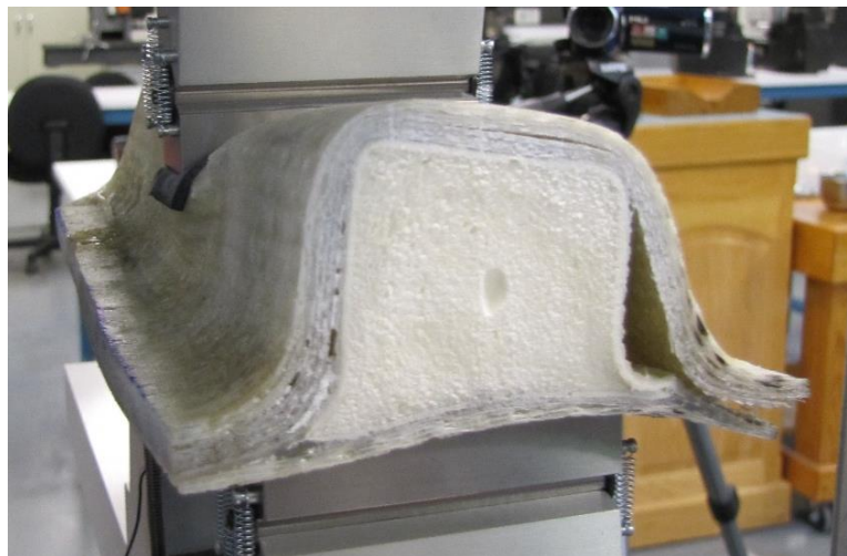
Figure 3.19: Unsymmetrical Deformation Caused by Splitting Between Shear Layers for Type 3
