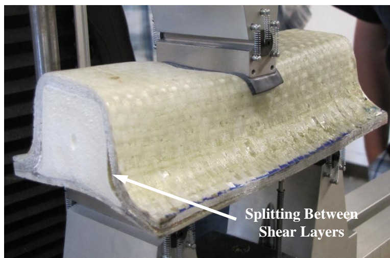
Figure 3.17: Initial Failure Due to Splitting Between Shear Layers for Type 3
