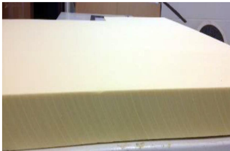
Figure 2.1: Type 1 Polyurethane Foam (PU RIGID)
