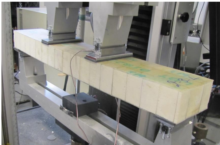
Figure 3.21: Type 2 (WEB-CORE) Sandwich Panel Specimen
